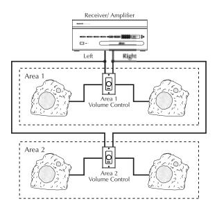
Figure 5 Two Zone Volume Control Wiring
